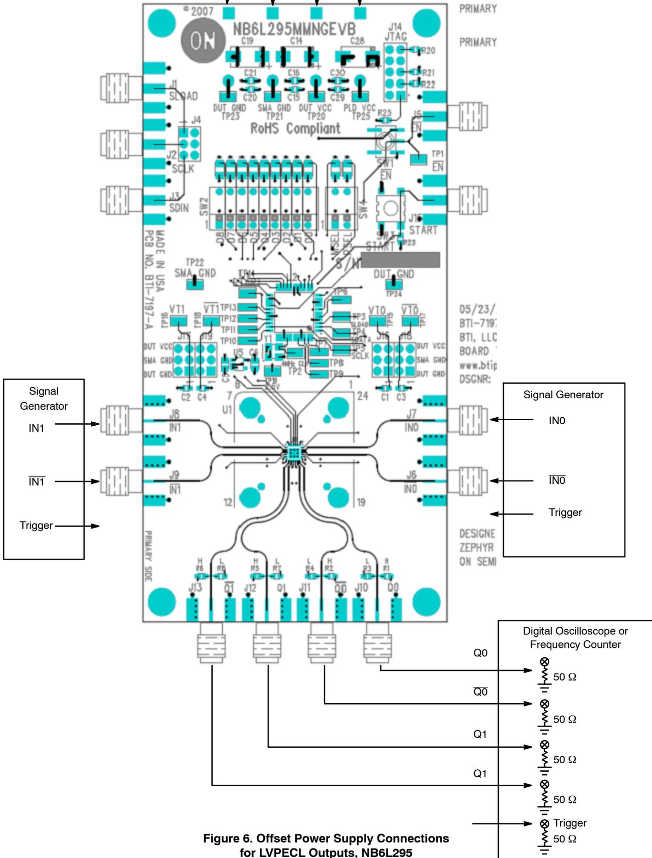
Figure 6. Offset Power Supply Connections for LVPECL Outputs, NB6L295
