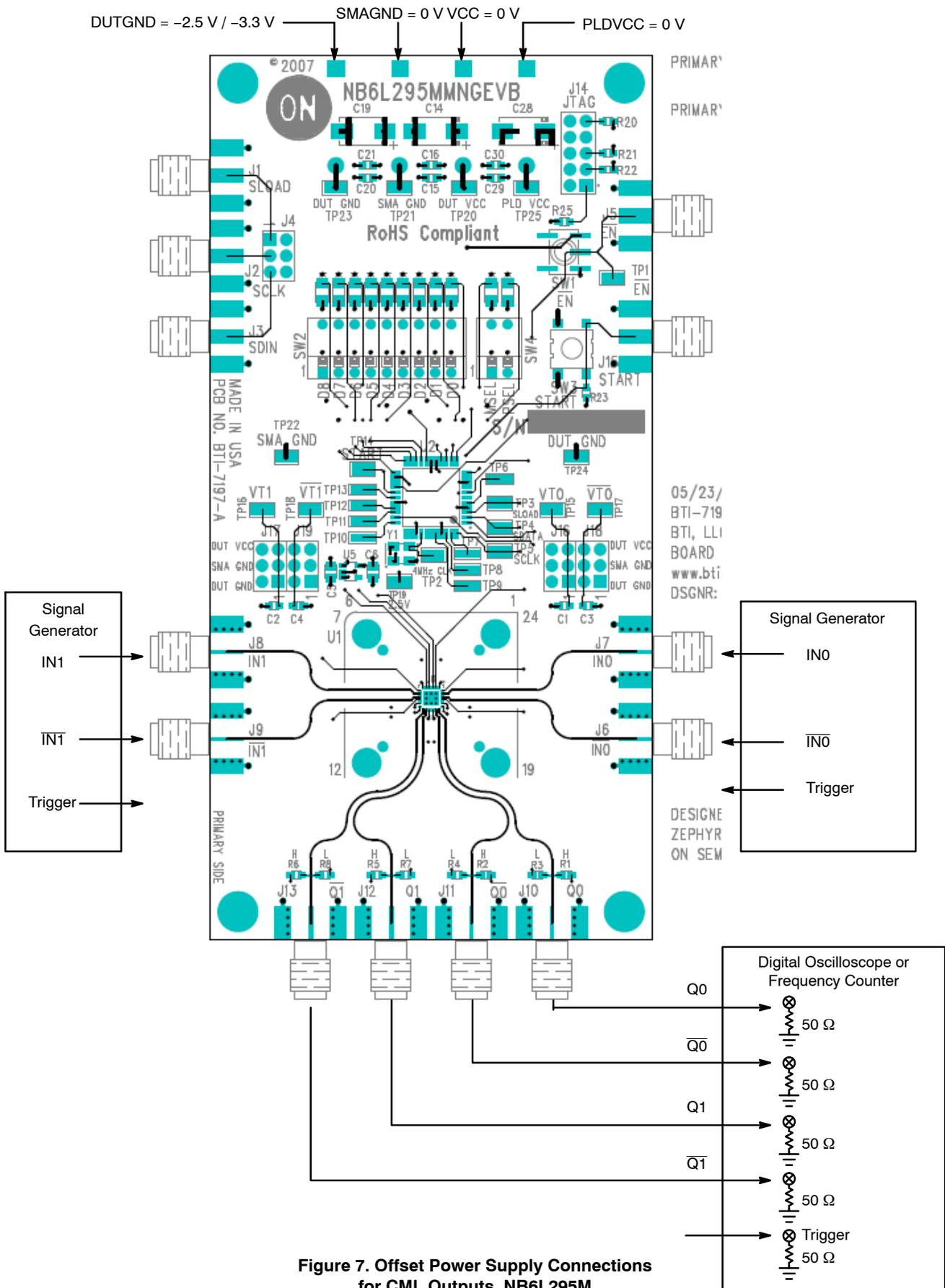
Figure 7. Offset Power Supply Connections for CML Outputs, NB6L295M
