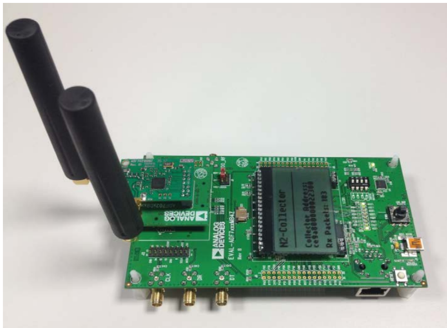
Figure 1. WM-Bus Development Kit (Includes Motherboard and Daughter Card)
