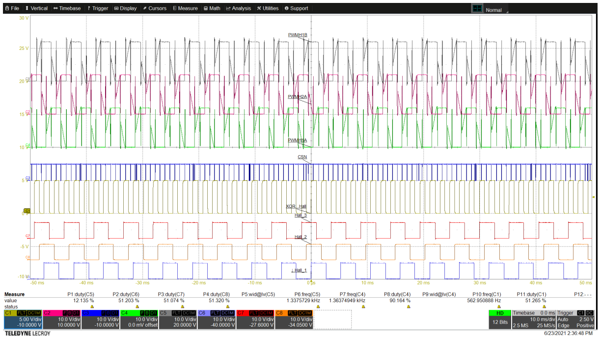
Figure 8. VBAT=12 V, 30 KHz PWM with 100% duty cycle (2 ms/div.)
