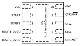
Figure 4-1. Pin Diagram DSK Package 10-Pin WSON
